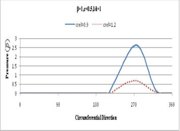
Fig:3- Pressure distributions in circumferential direction
