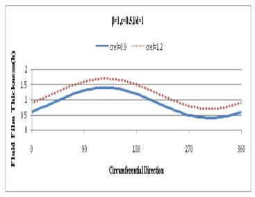
Fig: 5-Minimum film Thickness in circumferential direction
