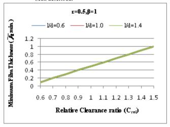
**Fig: 7-** Fluid film thickness ( $\overline{h}$ ) versus relative clearance for different bearing aspect ratio (l/d)
