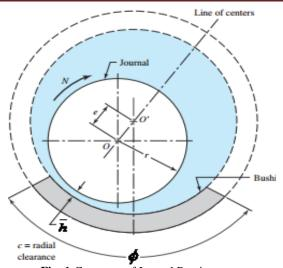
Fig: 1-Geometry of Journal Bearing
